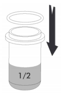
Install the O-ring seal (5) over the casing bowl (4). Seal should have a tight fit, if loose replace the O-ring seal. Fill the casing bowl (4) with clean diesel fuel no more than half way.
