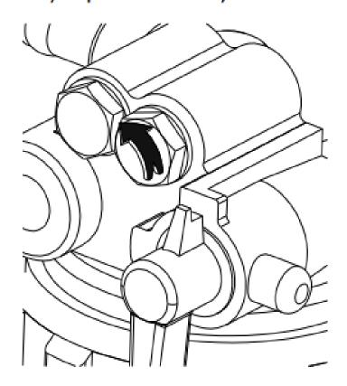
Loosen the vent screw (7) by ½ turn in the indicated direction. Vent screw should not be completely removed.
